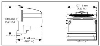
Figure 13. FP-CTR-502 Mechanical Dimensions
